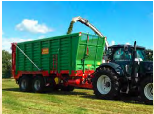
HAWE silage transport trailer SLW 45 TN, tandem axle volume: 42m 3 HAWE silage transport trailer SLW 45 TL, tandem axle volume: 45m 3
